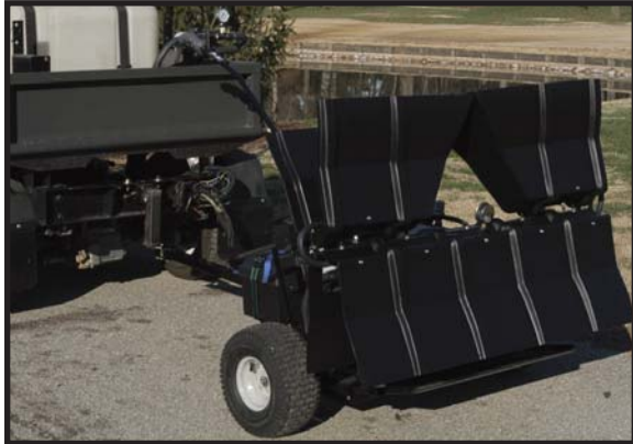
The outer wings and the handle fold up for compact transport.
