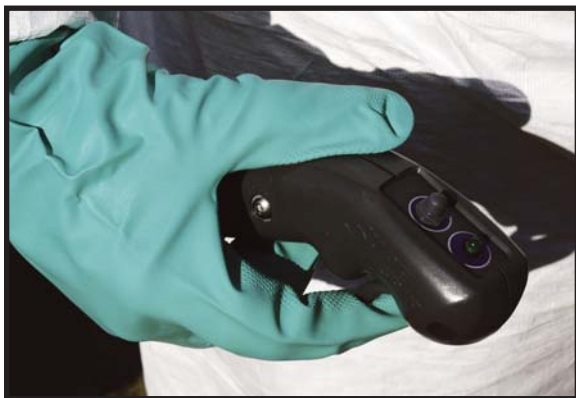
Convenient power drive switch and spray control switch are located at the operator's fingertips.
