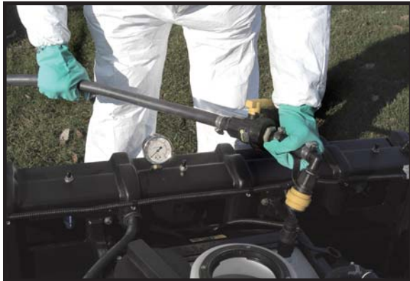
A dry lock fitting allows the operator to recharge the tank without exposure to the spray material.
