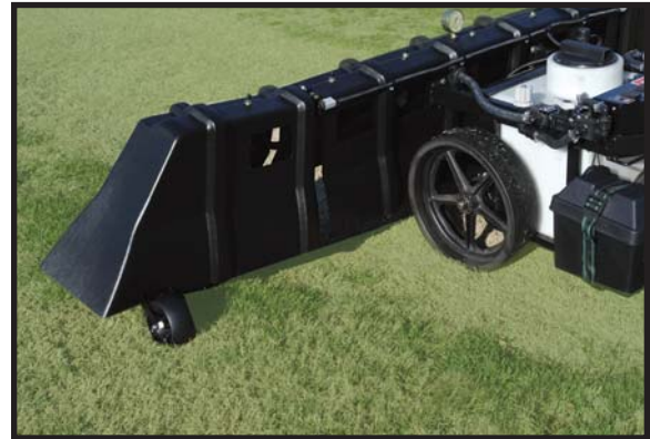
Nozzles remain at the desired height over rolling terrain with the floating outer sections.
