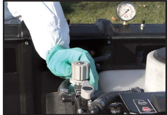
Calibration is easy by adjusting the pressure bypass valve.
