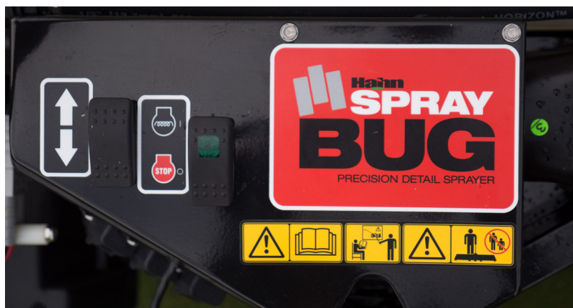
The Spray Bug can be operated in both directions with a flip of a switch.
