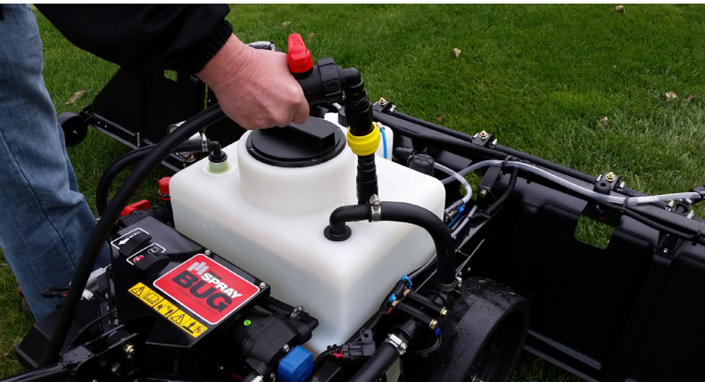
A dry lock fitting allows the operator to recharge the tank without exposure to the spray material.
